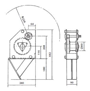
DIMENSION OF WINCH CLEVIS FOR WELDING TO RACK AND LOCO
