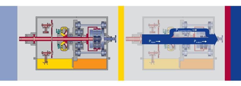
The Vorecon combines hydrodynamic components and a superimposed planetary gear within a single housing, perfectly combining the advantages of hydrodynamics and mechanics.
